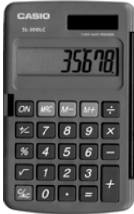
Figure 2: The Casio SL-300LC. Note the highly-visible self-advertising memory keys in the middle of the top row of buttons.
